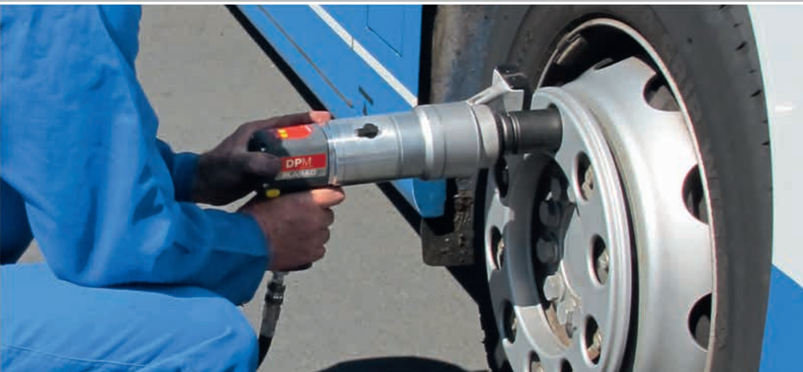
DP with angle drive: easy to use even in otherwise inaccessible places thanks to its low height. The pneumatic motor and handle freely rotate on the gearbox.
